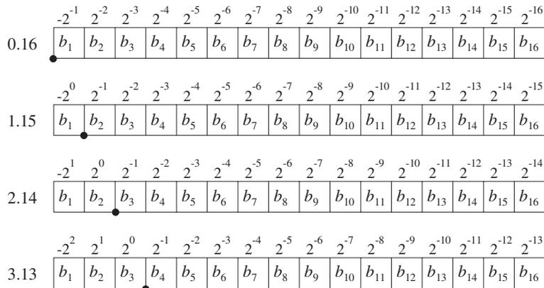
Fig. 2.1 Bit weights for 0.16, 1.15, 2.14, and 3.13 formats.
