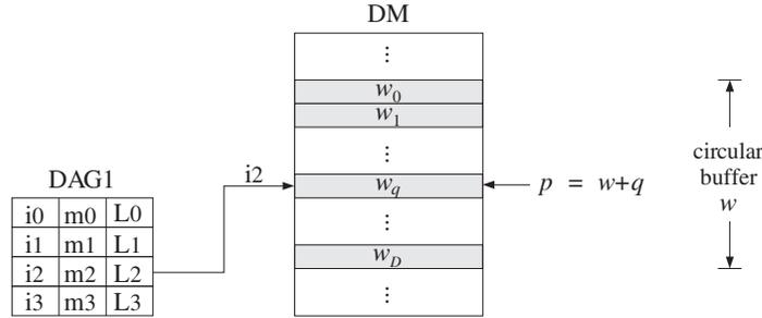
Fig. 3.2 DAG pointer into a circular delay-line buffer.
