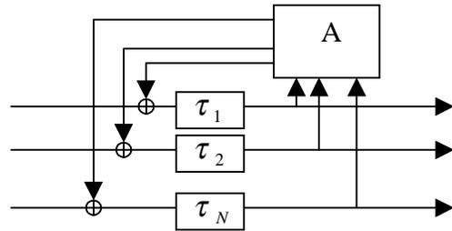
Figure 1. ‘Feedback Delay Network’ (FDN) topology
