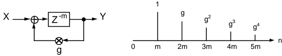
Figure 2.1 Comb filter flow diagram and impulse response.
