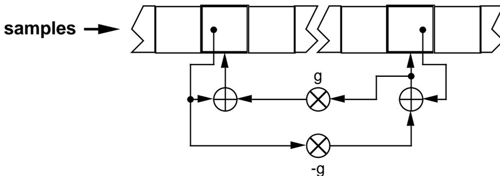
Figure 4.7 Allpass implementation using a sample delay line.
