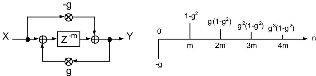
Figure 2.2 Allpass filter flow diagram and impulse response.
