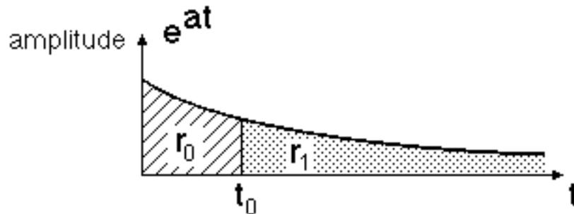
Figure 3.5 Amplitude envelope of idealized room response.
