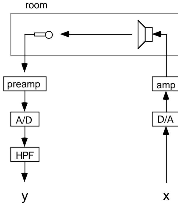
Figure 3.6 Block diagram of experimental cancellation setup.
