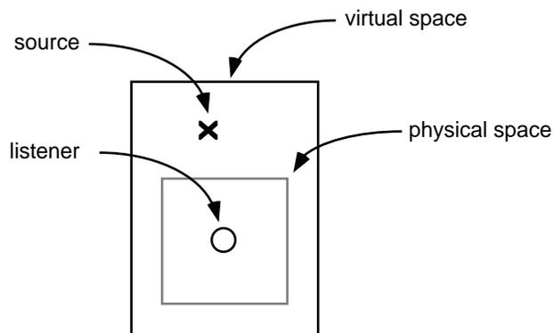
Figure 4.5 Rectangular virtual space and direct source location.
