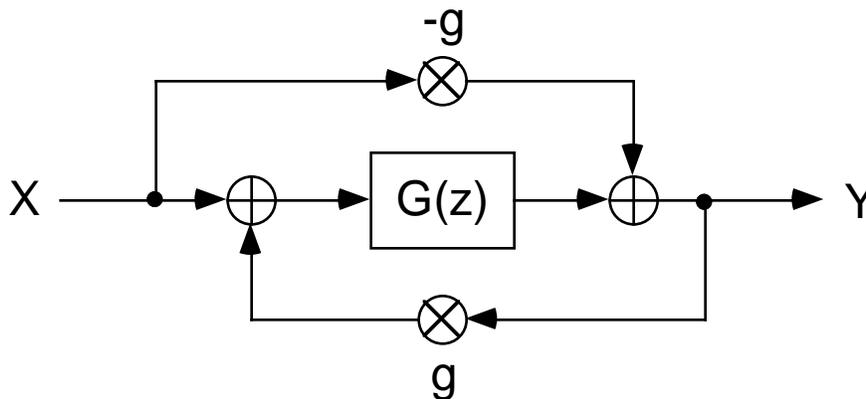
Figure 4.6 Allpass flow diagram.  $G(z)$  must be allpass.
